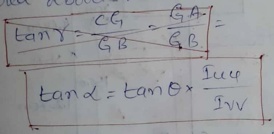
where  $\alpha$  is the angle of inclination of the neutral axis with respect to VV axis
