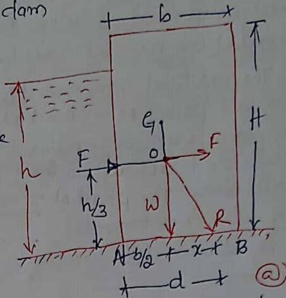
(ii) The weight  $W$  of the dam at the C.G. of the dam.
