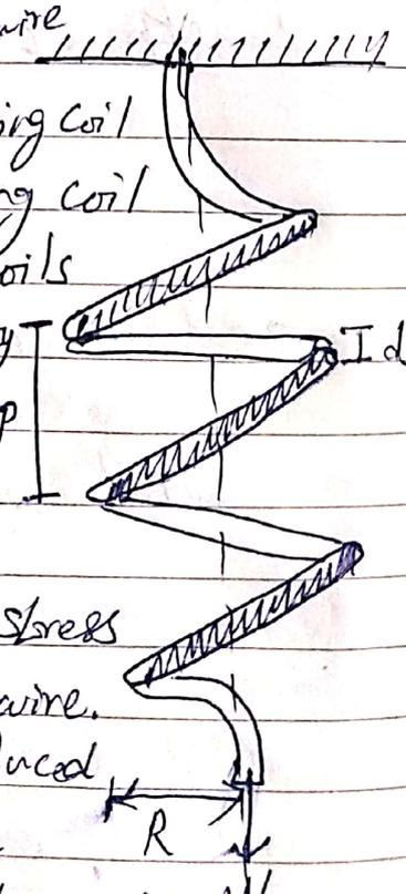
The load  $W$  will cause a moment  $WR$ . This moment may be resolved into the following two components,
