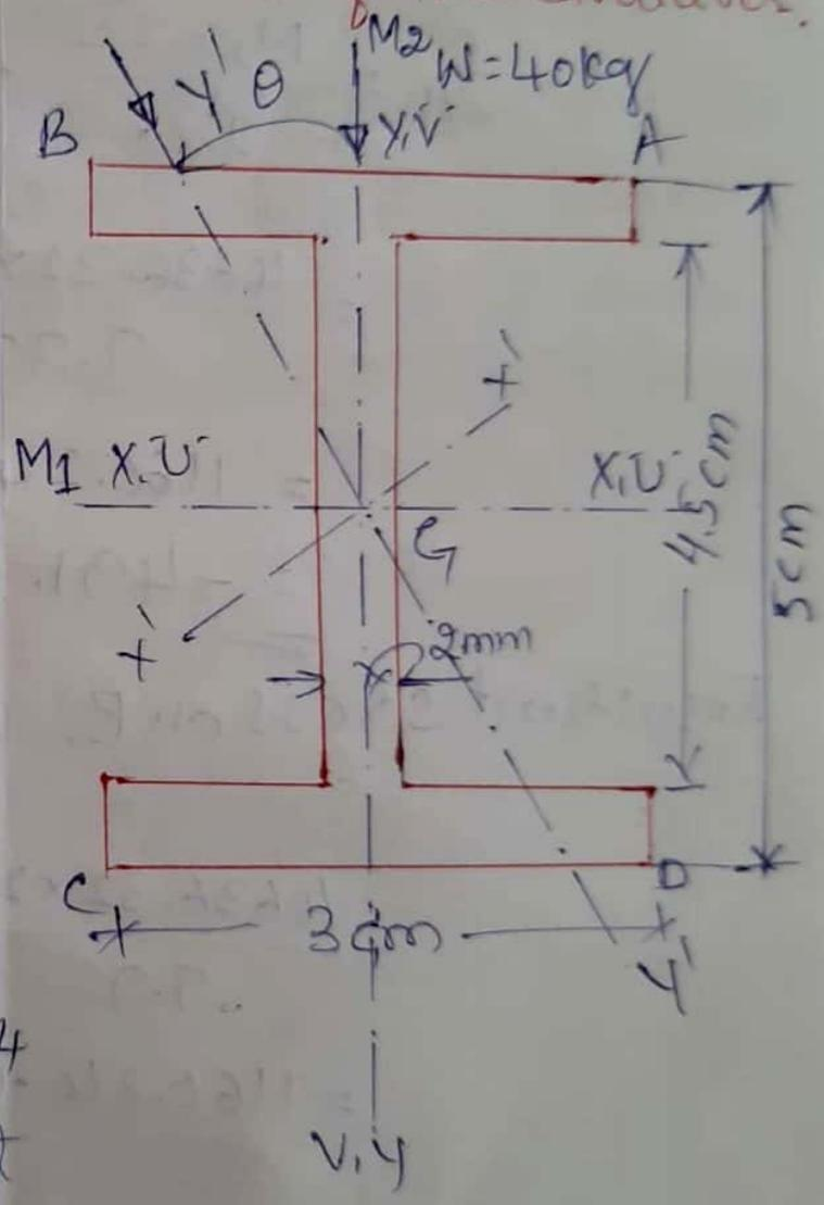
Due to bending moment  $M_1$ , there will be tensile stresses at points B and C and compressive stresses at points D and A.
