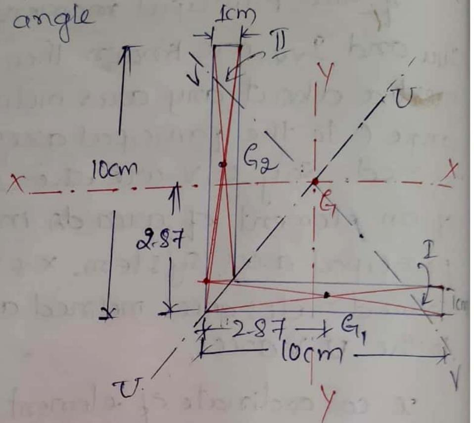
Let us consider the angle section in two positions I & II, as shown and determine the position of the centroid.
