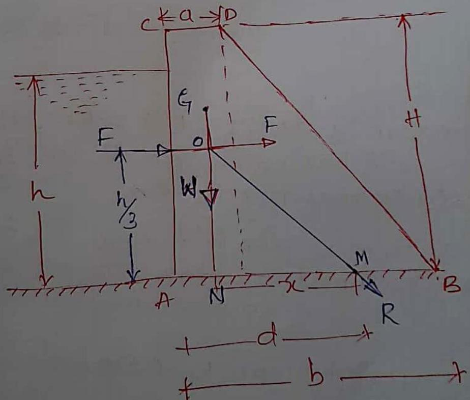
Fig shows a trapezoidal dam having water face vertical. Consider one metre length of the dam.
