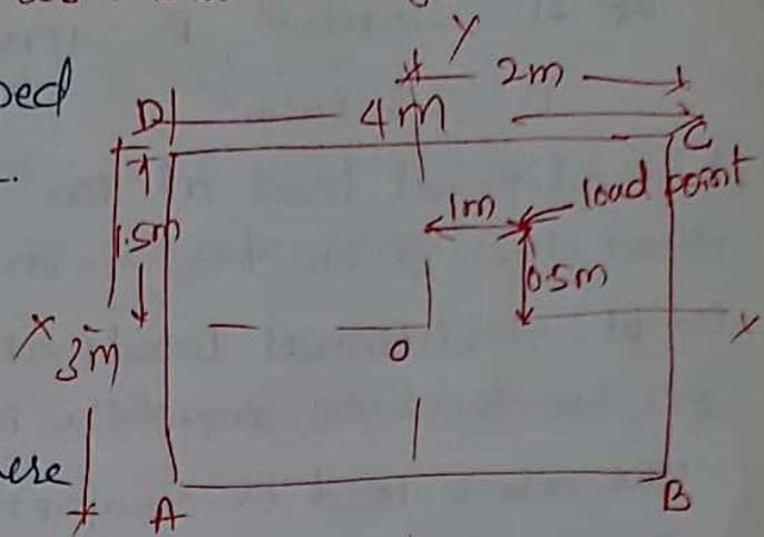
Sol<sup>n</sup>.  $b = 4\text{m}$ ,  $d = 3\text{m}$   $\therefore A = 4 \times 3 = 12\text{m}^2$
