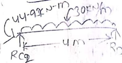
$$R_A = 48.595 \text{ kN} \approx 48.6 \text{ kN}$$
