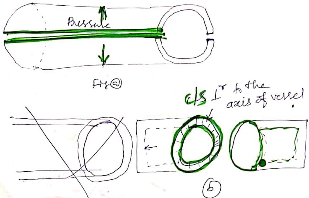
The forces, due to pressure of the fluid acting vertically upwards and downwards on the thin cylinder, tend to burst the cylinder (a).
