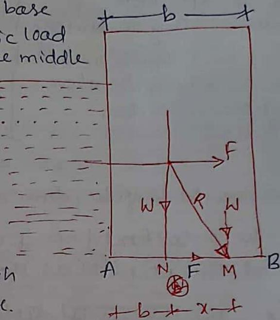
$\therefore$  Eccentricity of the vertical component  $W$  is equal to distance  $NM$  which is equal to  $x$  in this case.
