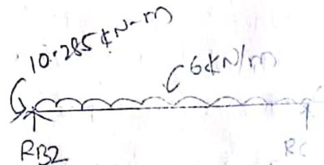
$$R_B = R_{B1} + R_{B2} \Rightarrow 12.858 + 14.57 \Rightarrow 27.428 \text{ kN}$$
