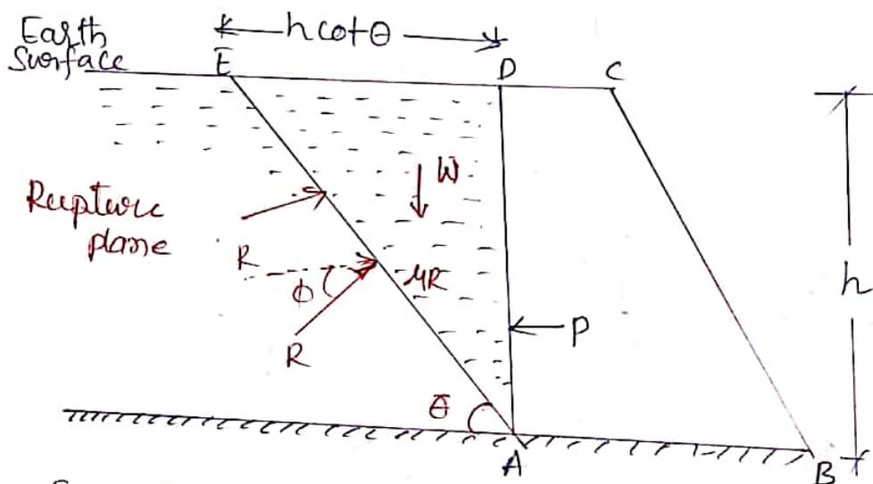
Fig shows a trapezoidal retaining wall ABCD retaining the earth upto a height 'h' on the vertical face AD. Let the earth surface is horizontal & it is in level with the top of the retaining wall.
