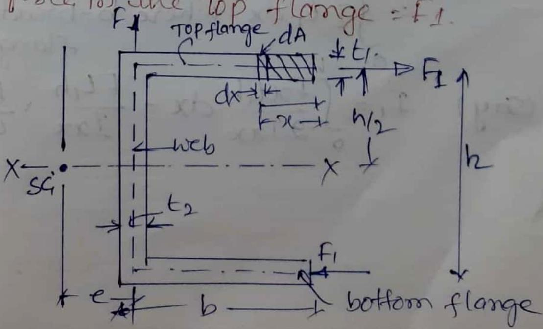
Shear stress in the flange at a distance of  $x$  from right hand edge.
