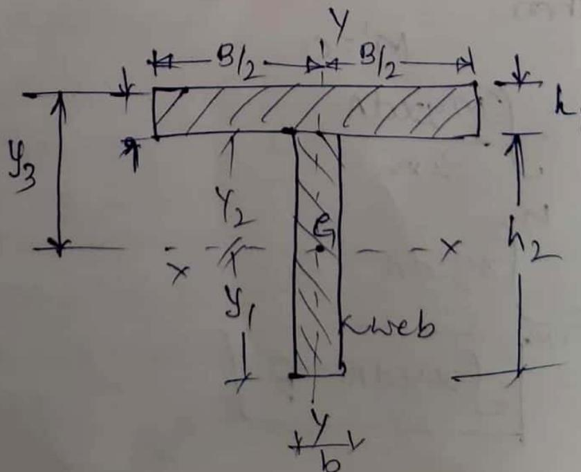
T-section with flange  $B \times h_1$  and web  $b \times h_2$ . The section is symmetrical about  $YY$  axis. Say  $G$  is the centroid the section on the axis  $YY$ , and  $XX$  &  $YY$  are the centroidal axes.
