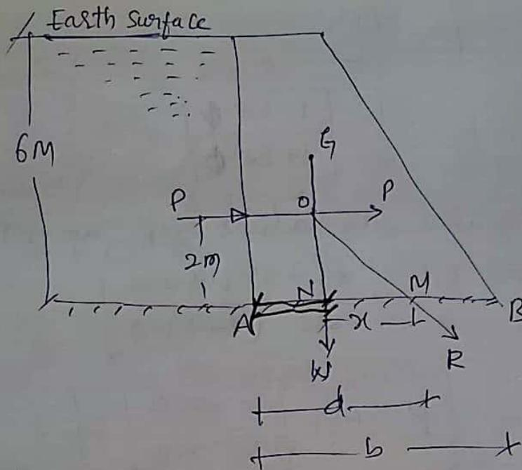
Consider one metre length of the retaining wall
