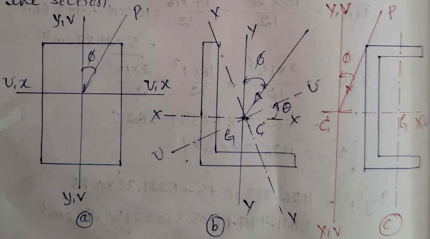
Fig (b) shows an angle section which does not have any axis of symmetry. Principal axes  $U'U'$  and  $V'V'$  are inclined to axes  $XX$  and  $YY$  at an angle  $\theta$ . Load line is inclined at an angle  $\phi$  to the vertical or at an angle  $(90 - \phi - \theta)$  to the axis  $U-U$ . Load line is passing through  $G$  (Centroid of the section) or  $C$  (Shear centre).
