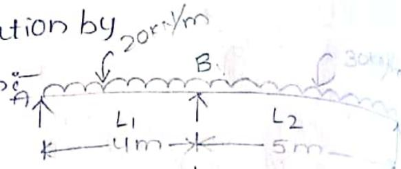
$$M_A L_1 + 2M_B (L_1 + L_2) + M_C L_2 + \frac{6a_1 x_1}{L_1} + \frac{6a_2 x_2}{L_2} = 0 \quad \text{--- (1)}$$
