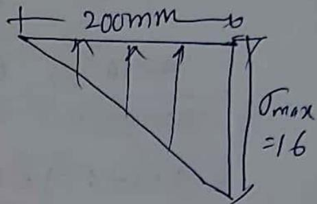
③ A rectangular column of width 200mm and of thickness 150mm carries a point load of 240kN at an eccentricity of 50mm then find the maximum and minimum stresses on the section. Also plot these stresses along the width of the section.
