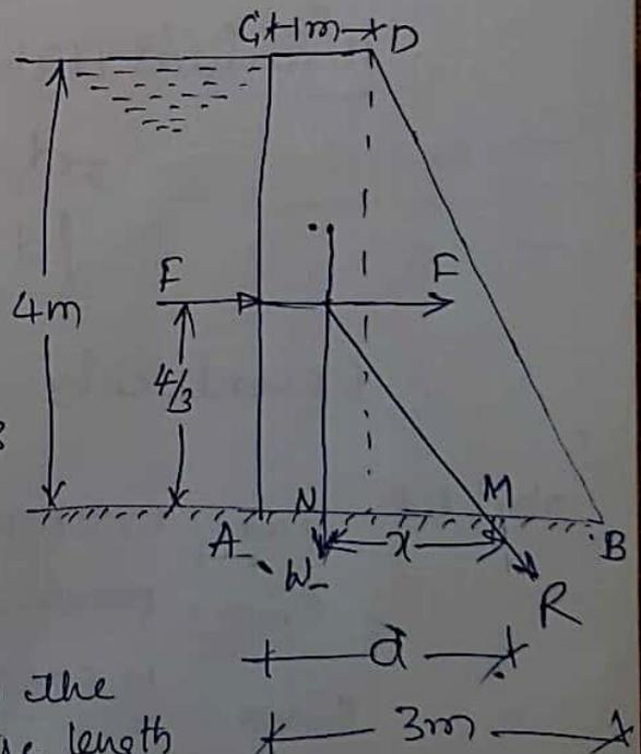
The weight of dam per metre length is given by.
