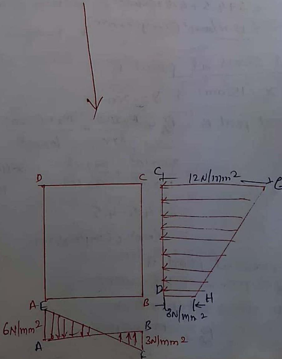
② A masonry pier of  $3\text{m} \times 4\text{m}$  supports a vertical load of  $80\text{kN}$  as shown in fig.
