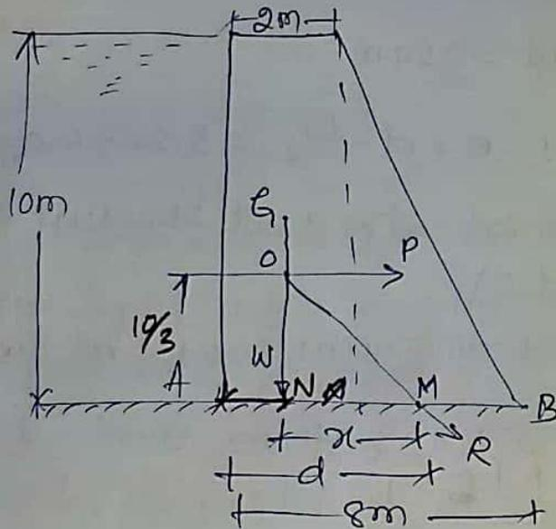
Thrust of earth on the vertical face of the wall is given by equation
