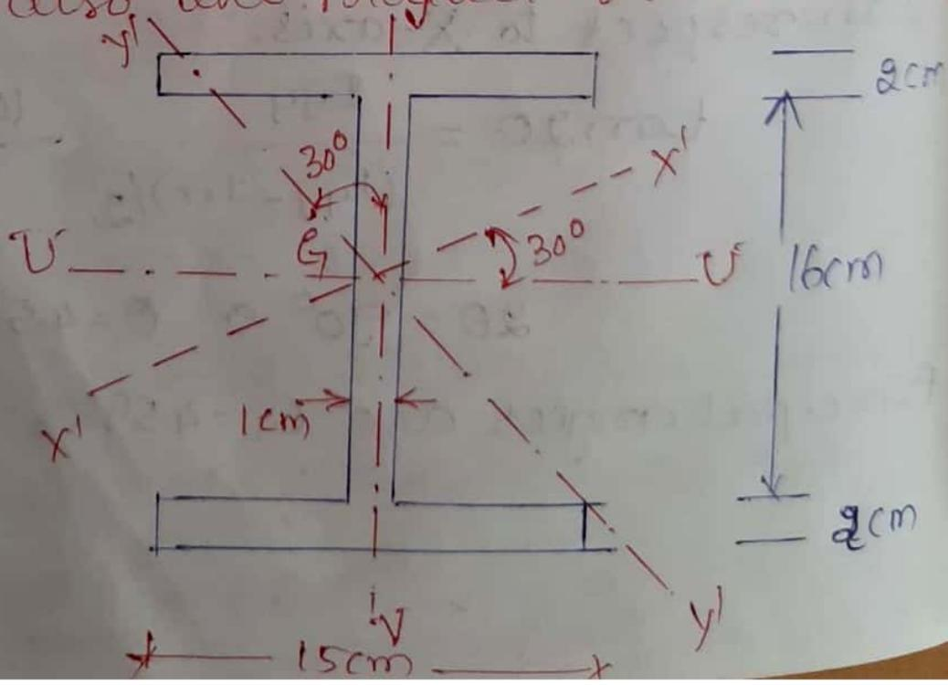
The I Section shown has two ~~axes~~ <sup>PAGE NO.</sup> of symmetry i.e., UU and VV passing ~~are~~ through the centroid G. therefore, these are the principal axes and  $I_{uu}$  &  $I_{vv}$  are the principal moments of Inertia. the angle of inclinations of UU and VV axes with respect  $x'x'$  and  $y'y'$  axes is  $\theta = 30^\circ$ .
