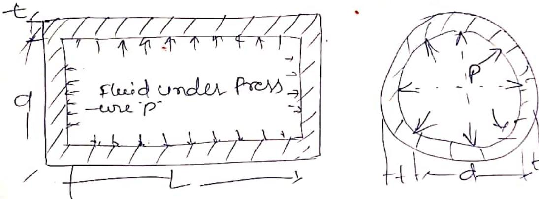
Fig shows a thin cylindrical vessel in which a fluid under pressure is stored.
